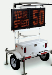
SpeedAlert 24 Radar Message Sign mounted on ATS5 Trailer
