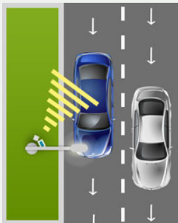
Unidirectional – Two incoming lanes with unit mounted on the side.
